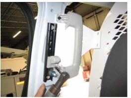
Install "B" pillar mounting bracket using bolts that hold grab handle. (*Re-installing the* grab handle is optional)
